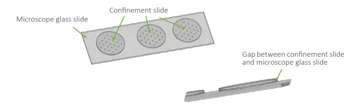
At least 1 h before the experiment, incubate the confinement coverslip and the suction cup in cell culture medium. Use the same medium that will be used for the experiment. The structured PDMS side of the slide should face upwards during incubation. Be careful not to lose the orientation of the coverslip.
