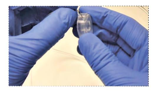
After connecting the suction cup to the autonomous pressure controller, you can verify that there are no leaks in your system by placing the suction cup on a clean surface (for example a container similar to the one used for your cells) and verifying that the piston moves down when you increase the pressure to -100 mbar. This should be visible as a divot in the center of the suction cup.
