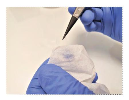
Place the confinement slide onto the piston of the cell confiner. The structured side faces up. The slide should stick naturally onto the piston. Please note that if the back side of the coverslip or the bottom side of the suction cup are not completely dry, they will not stick together and the confinement slide can be lost during your experiment.
