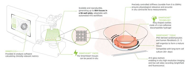
SmartHeart<sup>®</sup>'s design is compatible with in situ fluorescence imaging, allowing precise assessment of fixed tissue structures as well as live fluorescence imaging and optical mapping. Contractility and electrophysiology can be measured from the same videos, enabling the evaluation of excitation-contraction efficiency in the tissues.
