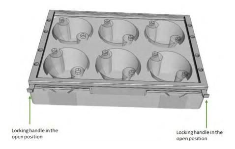
**8.** To lock the confiner, press the lid down on both left and right sides (as shown below, right image) and simultaneously lock the two handles by pushing them in. If you feel resistance, make sure the plate is assembled in the correct orientation as described in step 7.
