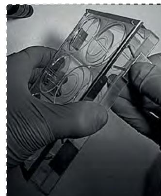
**7.** Place the lid on the top of the assembled holder. Allow it to be in the resting position, in which the springs hold the lid up.
