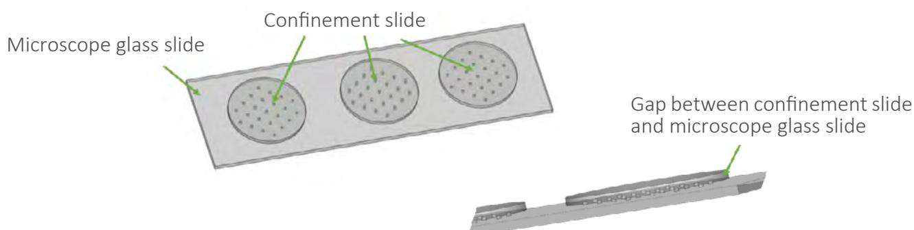
**5.** Place the confinement slide on the PDMS piston with the pillars facing up as depicted in the figure below. Make sure the slides are well centered on the pistons to avoid breaking the slides once in contact with the inner circle on the bottom of the plate. Avoid creating air bubbles between the PDMS piston and the glass coverslip.
