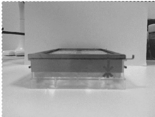
The tilted part of the plate holder should be facing the front when you assemble the lid and the holder.
