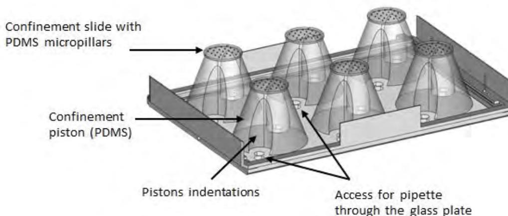
*The PDMS is usually sticky, enabling it to be attached to glass very easily. The holes in the lid (access for pipette through the glass plate) can be used to pipette media, aspirate it, etc. The holes can be closed with the white caps provided in the kit. If you find it difficult to remove the caps, please use tweezers to do so.*
