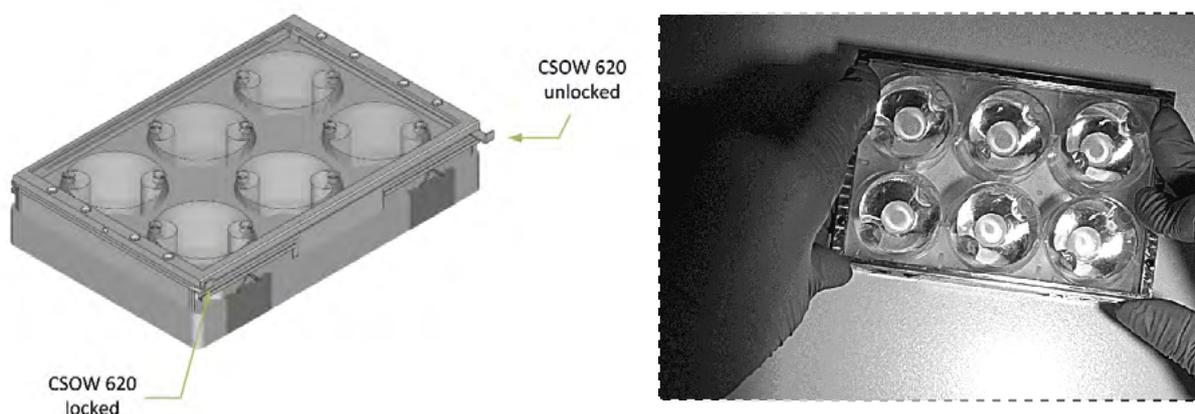
**9.** To unlock the confiner, gently pull the locking handles out and let the lid come up. If it does not come up naturally, gently move it upwards.
