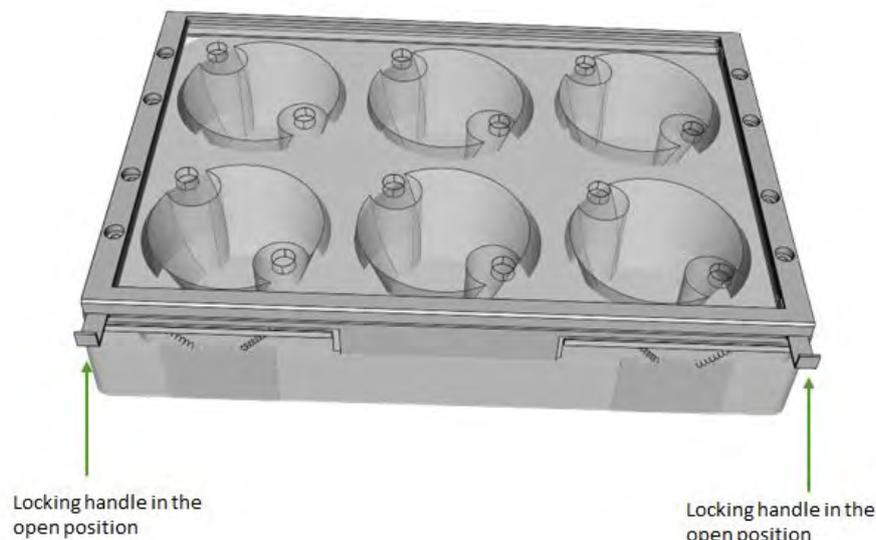
**8.** To lock the confiner, press the lid down on both left and right sides (as shown below, right image) and simultaneously lock the two handles by pushing them in. If you feel resistance, make sure the plate is assembled in the correct orientation as described in step 7.
