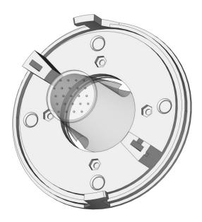
The PDMS is usually sticky, enabling it to be attached to the glass very easily. The piston can be cleaned and sterilized with ethanol 70%. If the PDMS piston has particles of dust, you can use the tape provided in the kit to remove them previously to sterilizing it. Do not forget to align the indentations of the piston with the holes existing in the glass part of the lid. These can be used to pipette media, aspirate it, etc. The holes can be closed with the caps provided in the kit.
