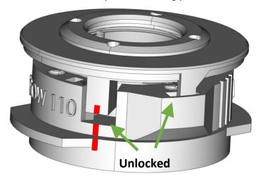
**8.** To confine the cells, from the unlock position, gently press the lid down and then rotate clockwise. At this point, your cells are confined.
