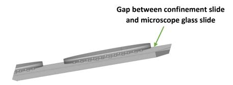
**3.** Place the confinement slide on the PDMS piston with the pillars facing up as depicted in the figure bellow:
