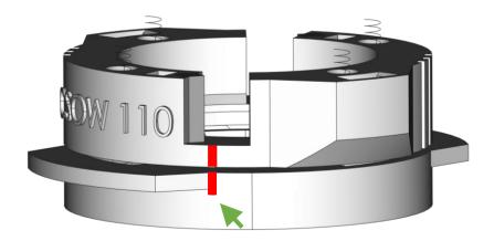
7. Put the lid on the top of the petri dish holder already assembled. Align the mark (here highlighted in red) in the lid with the bottom ones. There are two positions here, one locked and the other unlocked. When the lid is locked it means you are confining your cells.
